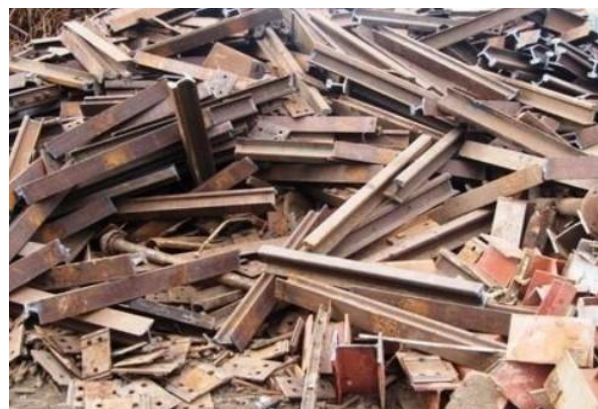
Heavy Melting Steel #1 (HMS1) is a commonly used designation of steel scrap defined by the Institute of Scrap Recycling Industries
